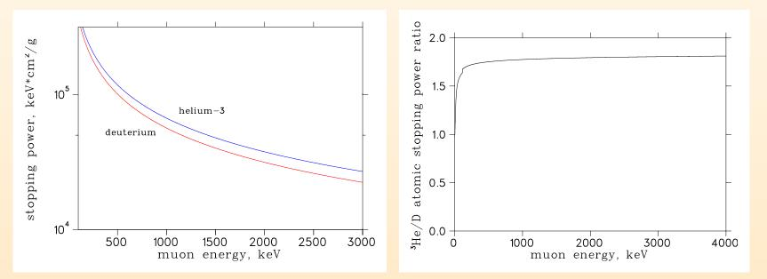
Calculated stopping powers (using data of J.F.Ziegler et al., The Stopping..., Pergamon Press, N.Y., 1985)
